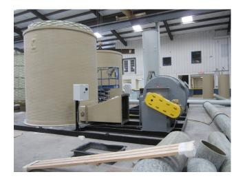
All components of these two odor control systems were manufactured and assembled in the ECS manufacturing facility – with the exception of the control panel, fan and flexible connectors which were outsourced and assembled prior to delivery.
